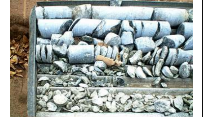
Photo 4. An example of drill core with disking and borehole breakout
