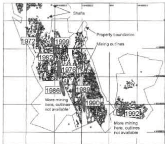
Figure 1. The distribution of tremors > magnitude 4.6 in the Welkom gold field. The outlines of mining faces shown are those along Basal reef, that dips at an average of 20° to the east and is mined at an average depth of 2000 m below surface. All these tremors had a normal slip mechanism. The ellipses indicate the approximate sizes and shapes of the areas of significant co-seismic displacement (van Aswegen 3 ). The co-ordinate grid spacing is 5 km
